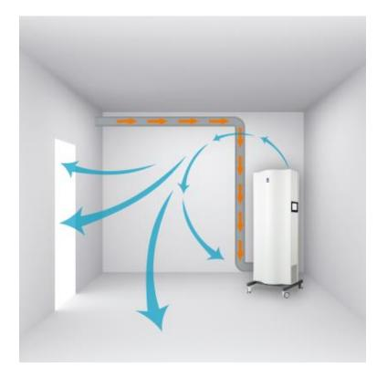
The supply air of the central ventilation is led into the room through the Genano air purifier The device is capable of controlling the positive pressure difference, which should be 5–10 Pa relative to adjacent spaces. To obtain maximal results, the supply air should be at least 20 % more than the exhaust air and the air leakage should be under control.
